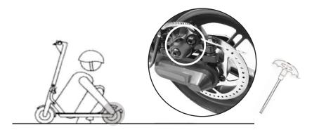
If you feel any vibrations in the control rod, it is advisable to tighten the 2 screws located at the base of the locking/unlocking mechanism with an M6 Allen key (not included).
