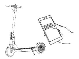
2. Press the power button on the electric scooter. Make sure GPS is enabled, the search for available Bluetooth devices will start automatically. Launch the App.
